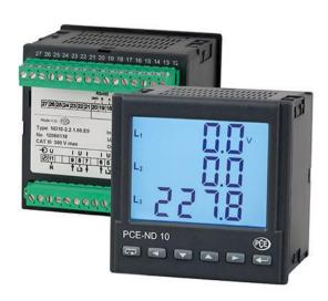
Digital indicator PCE-ND10 for permanent installation / Lighted 3.5 " display / 2 alarm outputs / impulse output / Modbus RTU interface / IP 656 front / phase recognition / measurement and display of power, voltage, power rating, efficiency factor, phase angle...
