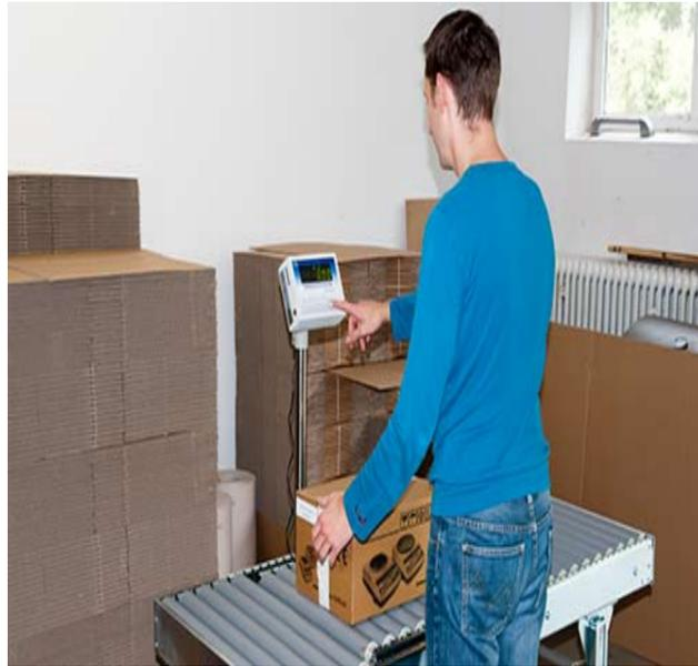
**RollerScale up to max. 30kg - 150 kg / bi-directional RS-232 interface /**
