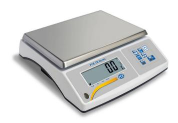
Reasonablypriced Counting Scale up to 30 kg / accuracy down to 0.05 g / operation by battery possible / bi-directional RS232 interface /platform size  $300 \times 210 \text{ mm}$  / optionally purchasable: LAN, Wi-Fi, 4-20mA, 0-10 V or 3 potential-free contacts
