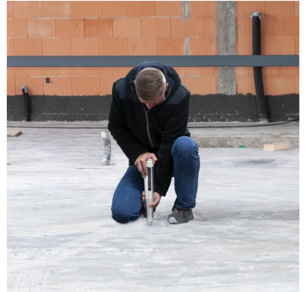
**Concrete test hammer based on the Schmidt principle / to determine concrete strength / high impact energy / quick and easy operation / for high-performance concrete**
