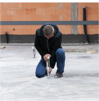
Concrete test hammer based on the Schmidt principle / to determine concrete strength / high impact energy / quick and easy operation / for high-performance concrete
