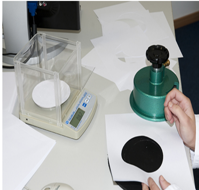
LAB Scale for Paper Basis Weight PCE-DMS 200-ICA incl. ISO calibration certificate 10 cm round pan for weighing 11 cm circle cut samples
