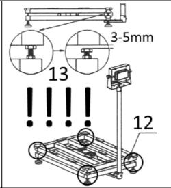
Finally, the balance must be aligned horizontally. To do this, turn the adjustable feet (14) of the weighing platform until the level indicator (15) shows a level position and the balance stands stably.
