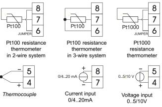
Fig.4. Connection of input signals.
