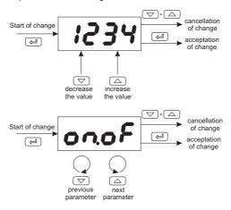
Fig.9. Setting change of numerical and textual parameters.
