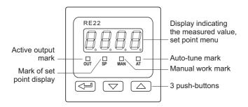
Fig.6. View of the controller frontal plate.
