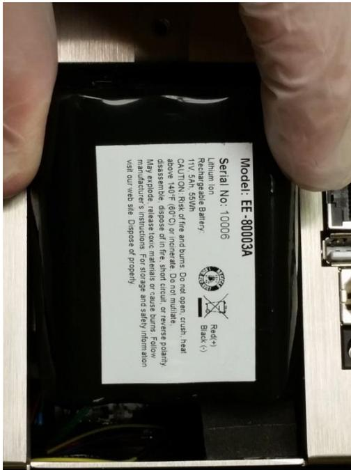
Step 5 – Carefully push battery into the compartment
