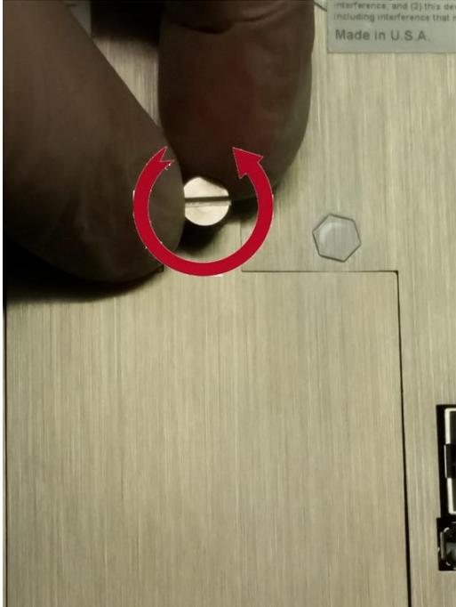
Step 1 – Loosen the Knurled Thumb-turn screw
