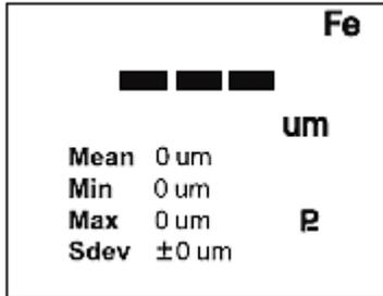
The **P** icon means that the thickness measured is beyond the measuring range or the meter has failed to measure.
