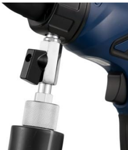
Borescope PCE-VE 250 with open shut-off valve
