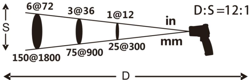
The farther the meter is away from the surface to be measured, the more space will be measured. If the distance-to-spot ratio is too large, undesired surfaces may be included in the measurement. This will cause incorrect readings.
