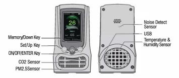
Set/Up Key: Long press to enter/exit the settings page; Short press to switch measurement displaying in measure page, or to turn on in settings/memory page.
