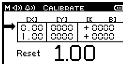
**Figure 6:** Calibrate Screen with Zero Measurement Complete
