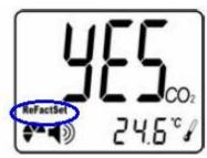
Using this function deletes all stored settings and sets the device back to factory default settings. This might be reasonable if the calibration has not been done properly, for example.
