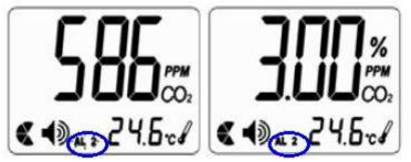
To adjust the AL2 threshold level, press the "Mode" key until "AL2" appears on the display and press "Enter" to confirm. Now you can switch between the available options by pressing the "Mode" key. The following options are available: 1.5 %, 2 %, 2.5 %, 3 %, 3.5 %, 4 %. Select the desired option and press the "Enter" key to confirm.
