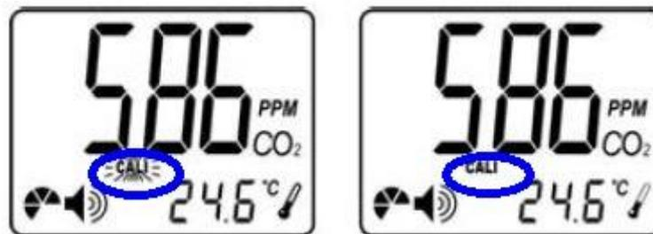
The gas detector should be calibrated at least every two years. To do so, you can use the ambient air outdoors. The housing needs about 10 minutes to acclimate. Wait until the CO<sub>2</sub> reading on the display is stable. The display should indicate between 380 and 420 ppm.
