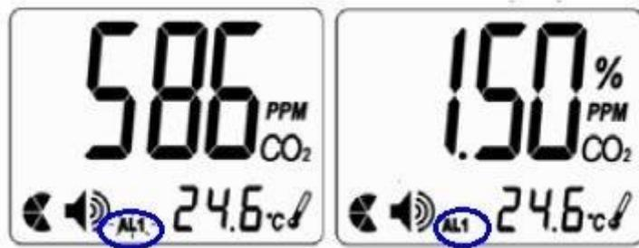
To adjust the AL1 threshold level, press the “Mode” key until “AL1” appears on the display and press “Enter” to confirm. Now you can switch between the available options by pressing the “Mode” key. The following options are available: 0.5 %, 1 %, 1.5 %, 2 %. Select the desired option and press the “Enter” key to confirm.
