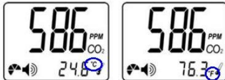
To switch between “°C” and “°F”, press the “Enter” key.
