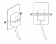
Connect the mains adaptor to the wall socket. Attach the elastic safety strip to the power plug by using screws and wall plugs. The strip should sit so tight that the plug cannot be pulled out of the socket without using mechanical tools. Once the mains adaptor is connected to the power source, the Sensor unit and the remote display unit start monitoring.
