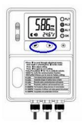
The gas detector has an automatic lock function to prevent the settings from being changed unintentionally. If you wish to adjust the settings you have to unlock the device first. To do so, press and hold the "Mode" key and the "Enter" key at the same time for 5 seconds. Now the device is unlocked and you can change the settings. After 30 minutes, the device will be locked again. To activate the lock function manually, press and hold the "Mode" and "Enter" key once again for 5 seconds.
