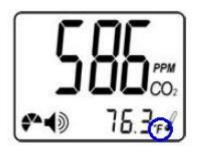
To switch between "°C" and "°F", press the "Enter" key.
