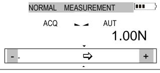
When ACQ indication is turned on, *MEM* key starts storing measurements in equal time intervals.
