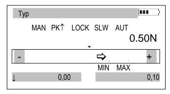
Changing actual force value indication into peak value measurement is done by pressing PEAK key. Indication stabilization sign changes into LOCK sign and force meter changes mode into peak value for force in both directions. Pressing again PEAK key changes mode into one-direction peak value: first for pressure force  $(PK\uparrow)$  and after another PEAK pressing for pulling  $(PK\downarrow)$ , zeroing is done by  $\rightarrow 0\leftarrow$  key.
