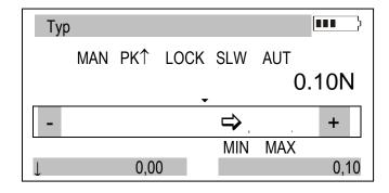
To perform the measurement, indicate the force direction using an arrow in the display's lower bar section and "+" (pressure) or "-" (pull force) symbol.
