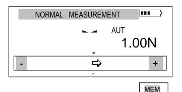
After pressing MEM key results are stored in buffer memory. Quantity of result in a 1 serie is set in *Memory/Setting/Quantity*.
