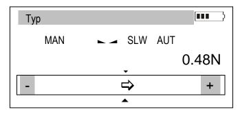
The force measurement is continuous. Display continuously indicates actual force value measured by meter. Force direction is signalized by an arrow in lower part of screen and a sign + (pressing force) or - (pulling force). Saving actual force indication to memory is done by pressing *MEM* key.
