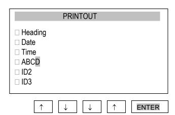
To enter the characters, select ID using ENTER and press  $\rightarrow$ . The characters are entered using the navigation keys  $\uparrow$  and  $\downarrow$ . To move the cursor to the consecutive positions, use  $\leftarrow$  and  $\rightarrow$ . To confirm the entered string, press ENTER. To delete character, enter space
