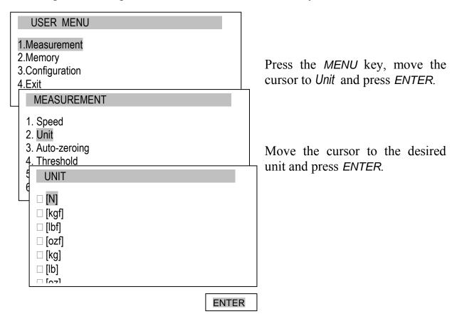
During mass measurement the force meter measures gravitation force and converts it to mass. Calculating force and mass unit is depended to gravitation force of the place of measurement. Default value is the producer gravitation value  $g = 9.81415 \text{m/s}^2$ . During very precise mass measurements ( $\pm 0.1\%$  of range) it is crucial to inscribe proper gravitation value of the measurement place (*Calibration* options).
