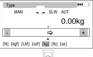
By pressing several times cursor is moved between different units until the proper one is chosen.
