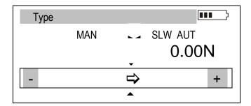
Place the gauge in the operating position, e.g. horizontal position (by laying it on a table). Turn on the gauge by pressing the *ON/OFF* key.
