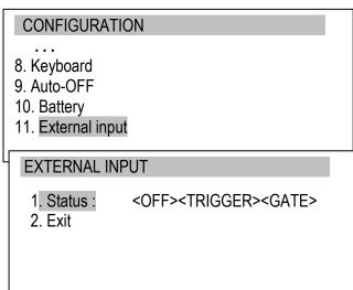
Using navigation keys and *ENTER* key choose *Configuration* option and then *External input*. Choose *Status* option and using  $\leftarrow$  and  $\rightarrow$  keys choose from:
