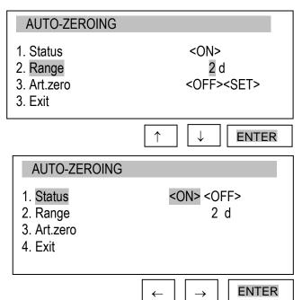
Additional option *Art.zero* enables to set device start zero to the value indicated before entering the *MENU*.
