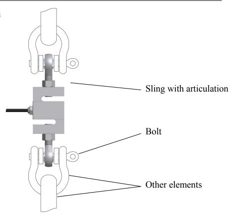
Bolt and other connection elements should sustain load even to 150% of force meter measurement range (150% Max). Moreover bolt should be matched to articulation diameter with tolerance -0.5mm and should be protected against moving in articulation. Articulation should be secured using pads against sharp slip.
