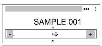
If indicator *MAN* (manual mode) is displayed, after pressing *MEM* key single measurement is stored.
