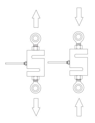
In case of force meters with external sensor force meter zeroing should be executed after mounting measurement post without any load.
