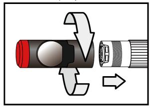
Step 4: Align the lateral LED opening of the mirror attachment in a way that the LEDs are uncovered. Step 5: Turn the assembly ring upwards in order to fix the mirror attachment.
