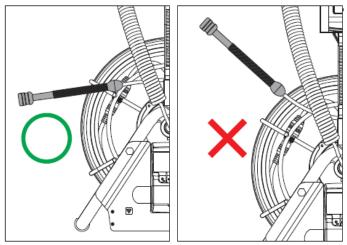
2. Pull out the camera cable horizontally. Do not pull it out in an angle larger than 45° to the camera head support.
