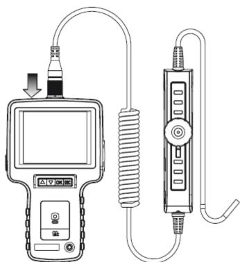
Connect the connecting cable to the display unit of the endoscope and screw it tightly. Make sure that the indication on the connector is on the upper side.
