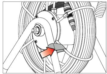
3. Once you have reached the desired cable length, fix the cable drum to prevent it from rolling out any further.
