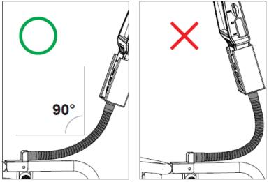
You can adjust the angle of the display support at any time, but do not use angles smaller than 90° cause this might damage the support.
