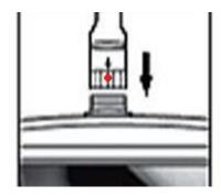
Connect the camera cable to the display unit and screw it tightly. Make sure that the indication on the connector is on the upper side (see picture above).
