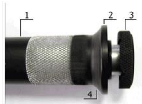
Figure 1a. UCI Probe U1 1 – Probe's body; 2 – Collapsible nozzle; 3 – Puck; 4 – Place for fingers
