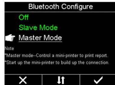
The meter will try to establish a Bluetooth connection with the printer. Wait for a few seconds. When the Bluetooth status LED glows continuously, this means that the meter is connected to the printer.
