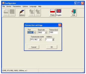
Fig.1 Connection configuration with the N24/25 meter
