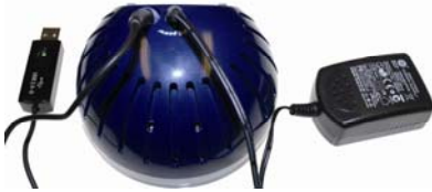
Fig. 5: Rear side of the Wöhler CDL 210 with USB cable and power supply
