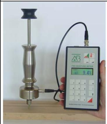
A photograph showing the FMD6 moisture meter connected to a probe. The probe is inserted into a piece of light-colored wood. The device's screen displays a moisture content of 9.4%. |
