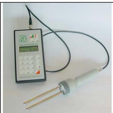
A photograph showing the FMD6 moisture meter and a probe. The probe has two long, thin metal needles. The device's screen displays a moisture content of 12.1%.                     |
