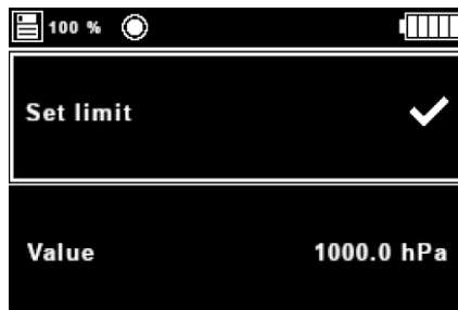
Fig. 58 Alert menu for pressure sensor
