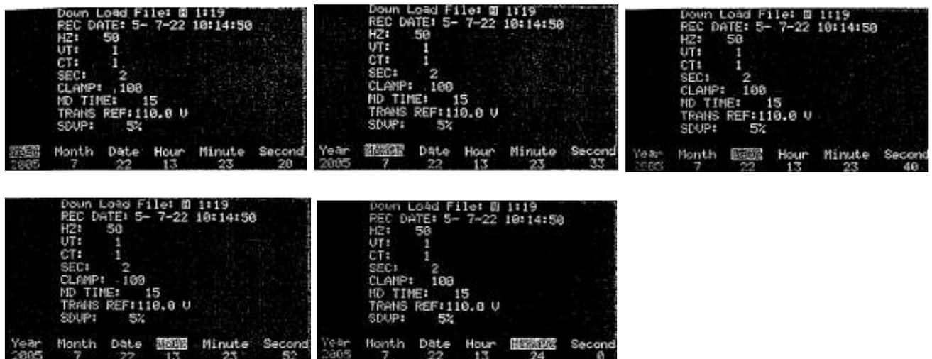
The following sequence of screenshots illustrates the process of adjusting the date and time:
