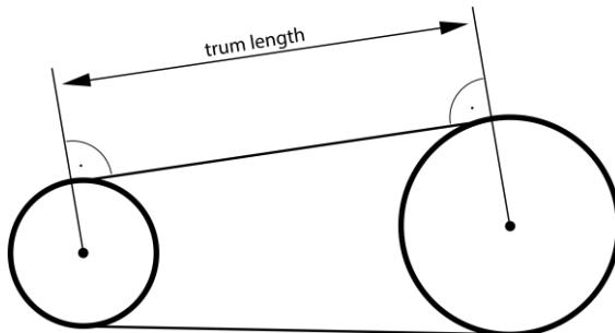
As a rule, the trum length can be measured directly on the belt. Measure the length described above (trum length) and enter it in the "Force" menu as the length. Sometimes it is not possible to measure this length - then you can determine the length using the following formula:
