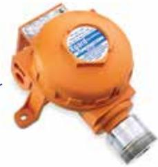
Flameproof high temperature (up to 150°C) catalytic bead type detector with mV bridge output.
