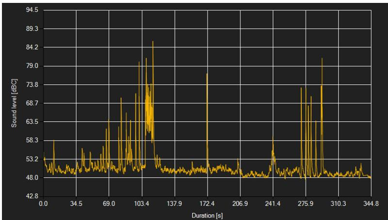
Moving the mouse cursor to a point in the displayed line makes a small information window with the data (time and unit) of the currently selected measurement value pop up after a short time.
