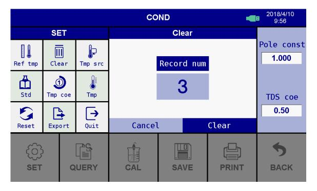
c) The source of temperature: "automatic" and "manual" two modes; according to the temperature source, such as the following diagram, the selection is or automatically press the set to save, by cancellation return.
