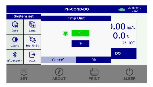
e) Bluetooth settings: connect to Bluetooth printer or mobile phone APP. According to the Bluetooth settings, you can choose to connect the Bluetooth printer or the phone APP, enter the authorization code, press the confirm save settings, press cancel to return.
