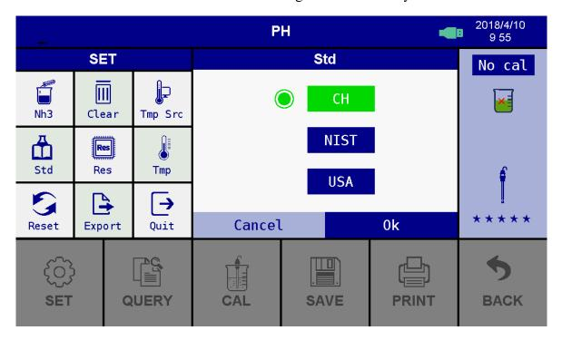
e) Resolution: 0.1pH and 0.01pH; according to the resolution, select the appropriate resolution as shown below, press the confirmation save settings and cancel the return.
