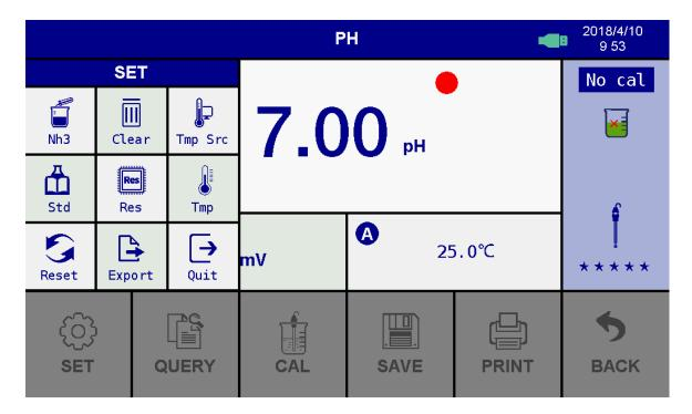
a) Adding ammonia compensation: "no compensation", "pure water compensation", "ammonia compensation" three modes; according to the addition of ammonia compensation into the following diagram, according to the determination of the storage settings, by cancellations return.
