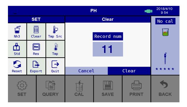
c) The source of temperature: "automatic" and "manual" two modes; according to the temperature source, such as the following diagram, the selection is or automatically press the set to save, by cancellation return.
