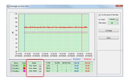
For the different acoustic parameters the average mode would be different. As shown in the red frame above, the options of the average mode could be: Exp. Mean, Lin. Mean, Maximum, and Minimum.
