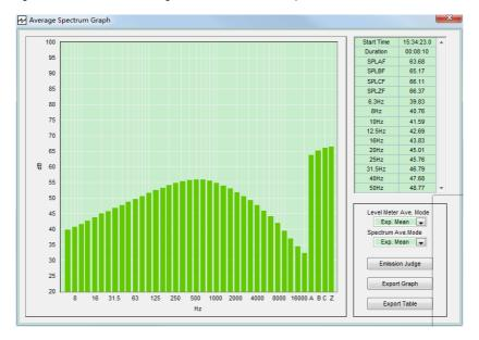
The average mode of the overall sound level and the spectrum can be set respectively. The graph and the table will be rewritten automatically according to the average mode. The
