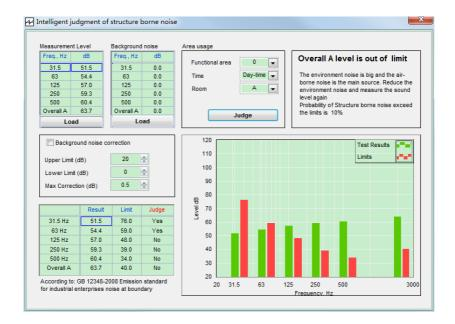
As shown above, the average spectrum of 31.5Hz to 500Hz will be input to the upper-left table, Click **<Judge>** after the Functional area is affirmed, Software will evaluate the structure borne noise inside according to GB12348-2008.
