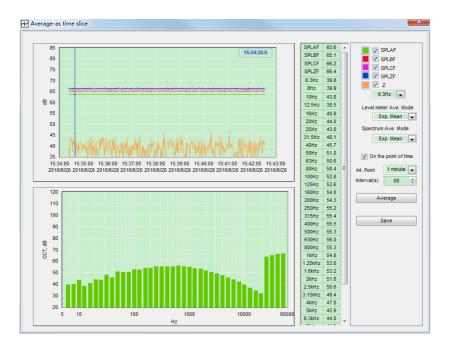
As described in 5.4.2, the average time slice is defined by **Interval(s)**, which can be input directly, or chosen by the **Int. Point**. The use of time slice has two ways: **On the point of Time** or **not**. The average mode of the overall sound level and the spectrum can be set respectively. The options of the average mode could be: Exp. Mean, Lin. Mean, Maximum, and Minimum.
