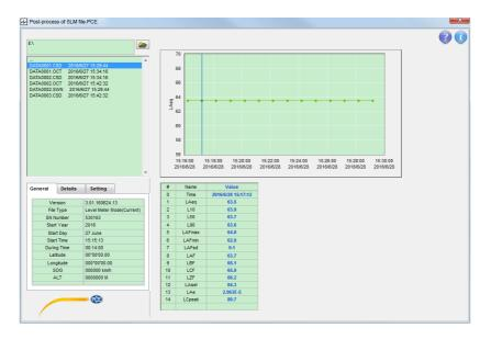
The figure above is the Level Meter display mode of CSD file. The CSD files save 14 acoustic parameters at each time point. All these 14 parameters of chosen time are shown in the table below. Move the cursor of the graph can change the chosen time. The default curve's amplitude shown on the graph is the first defined acoustic parameter. Click the other row of table can change to the other acoustic parameter.
