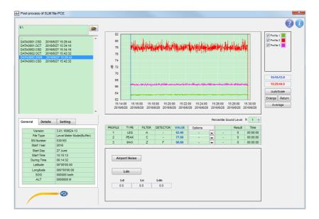
After the SWN file is read, the time curves will be shown in the graph, and the cursors will be fixed on both sides of the curve at first. The column" Value" in the table under the graph will show the reading of the blue cursor. Move the blue cursor to get the reading of the other time. Make sure that the blue cursor is earlier than the red cursor if you want to deal with the data between the two cursors.
