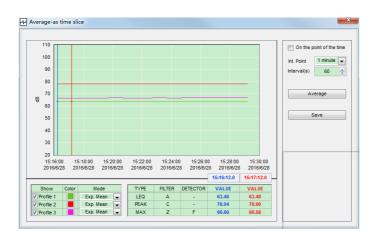
And if the "**On the point of time**" is checked, the average will be given when the time is the integral point. As the figure shown below, afert averaging the first result will be in 15:16:00, and the second result will be in 15:17:00...
