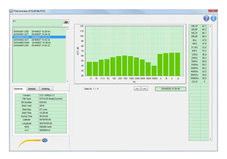
The Figure above is the OCTAVE display mode of CSD file. The CSD files save the spectrum of 1/1 OCTAVE or 1/3 OCTAVE at each time point. The values of the spectrum on the first time point are shown in the table on the right side, and the graph of the spectrum is shown in the middle.Click the key  $\langle \leftrightarrow \rangle$  or  $\langle \rightarrow \rangle$  to choose the other time point and the graph and the table will be changed accordingly.
